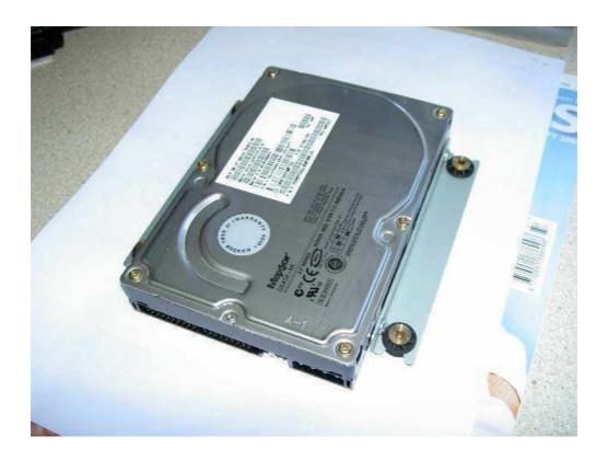
Set the new drives jumper to make it  $\square$  Cable Select  $\square$  as per the drive  $\square$  you removed  $\square$
