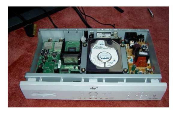
Unscrew and remove relse they will fall out the four screws in the rubber mounts either side of the hard drive Lift up and carefully unplug the IDE and Pin power cable from the hard drive Remember to take all necessary precautions to prevent damage by static discharge
