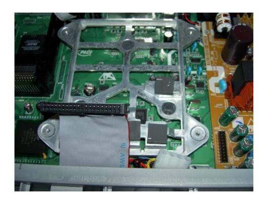
Make note of the four thermal transfer pads one out of site as IDE cable is in shot
