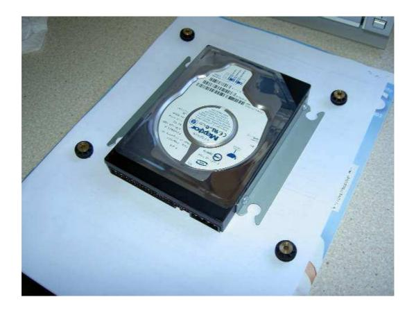
Take the hard disc assembly to a suitable clean antistatic work surface
