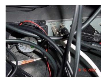
Here you can see a standard wolt computer power supply cooling fan fitted to extract hot air from the digibox and you don't even have to open up your box simply power the fan with a cheap power adaptor or even one of those spare mobile phone chargers you have lying around the house in
