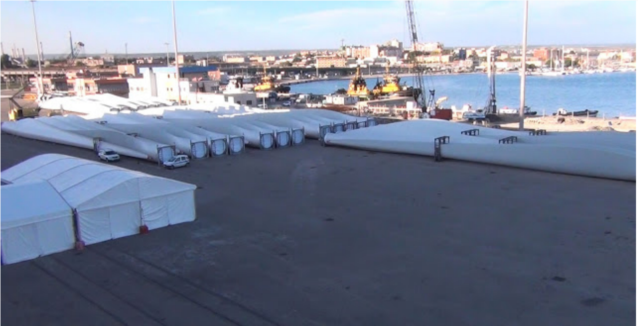
Sections of wind turbines laid out on the quay waiting for shipment
